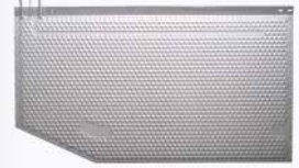
Heating blades in a drum for tobacco conditioning with steam, vibration transport channels for tobacco
